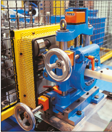
Digital indicators are responsible for aligning the tools within the "metal forming" process chain.
