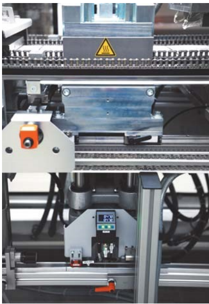
The stations mounted on guide rails can be adjusted easily and quickly on the Z.PACK – thanks to SIKO position indicators. (Photo credit: ZAHORANSKY AG)
