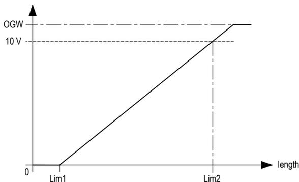
Fig. 6: signal sequence voltage output (e.g. 0-10 V)
