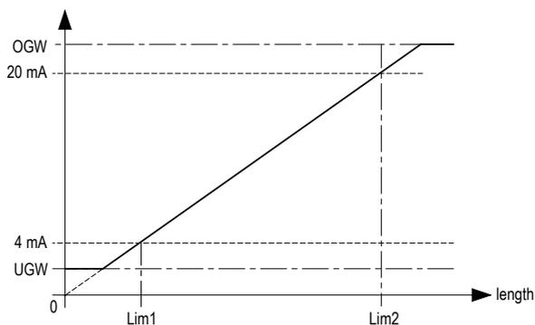
Fig. 7: signal sequence current output (e.g. 4-20 mA)
